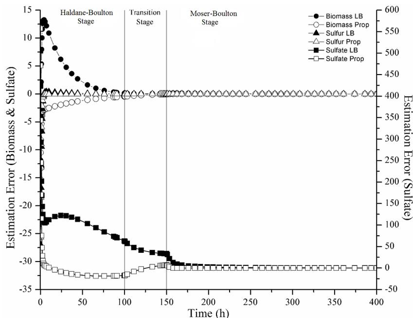
Figure 4. Estimation error for Sulfate (right axis), Biomass and Sulfur (left axis) concentrations for the Luenberger observer (black symbols) and the proposed observer (white symbols).
