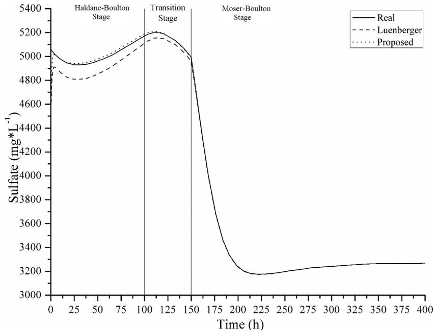
Figure 3. Simulation of the sulfate concentration consumption (continuous line) and the state observers (Luenberger observer, dashed line and the proposed observer, dotted line).
