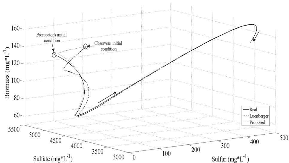
Figure 5. Phase portrait of state variables of the bioreactor (continuous line), the Luenberger (dashed line) and the proposed observers (dotted line).
