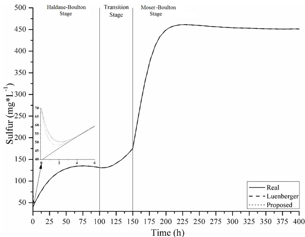
Figure 1. Simulation of the sulfide concentration production (continuous line) and the state observers (Luenberger observer, dashed line and the proposed observer, dotted line).
