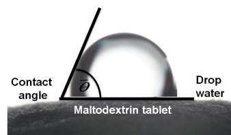
Fig. 1. Contact angle between water drop and maltodextrin tablet
