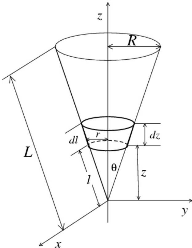
FIGURE 1. A hollow right circular cone with radius  $R$ , lateral length  $L$ , and uniform mass  $M$ . The cone's high is  $H = \sqrt{L^2 - R^2}$ . The figure also shows at the lateral distance  $l$ , measured from the cone's apex at the origin of the coordinate system, an infinitesimal ring of lateral length  $dl$  and radius  $r$ . Two useful geometrical relations among some of the dimensions shown in the figure are  $r = (R/L)l$  and  $r = (R/H)z$ .
