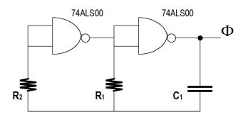
FIGURE 3. The RC2-NAND oscillator circuit.
