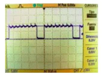
FIGURE 4. By lowering the bias voltage a spurious effect appears on the output response.
