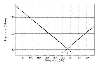
FIGURE 6. Spice simulation of the equivalent impedance versus frequency.
