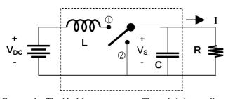
FIGURE 1. The ideal boost converter. The switch is actually a semiconductor device.
