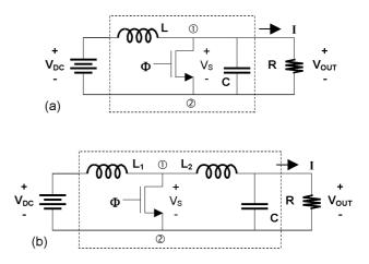
FIGURE 2. The boost converter using a MOS transistor as a nondissipative switch (a). Including a second inductor,  $L_2$ , harmonics are eliminated (b).
