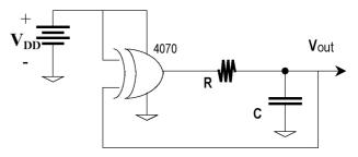
FIGURE 8. EX-OR gate is also useful in developing an oscillator circuit. The bias of the circuit presented here must satisfy the condition  $3V \le V_{DD} \le 15V$  for correct operation.
