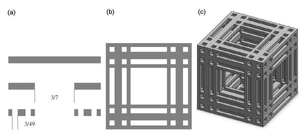
FIGURE 4. Generation process of Cantor Tartan  $\mathcal{CT}_3$ . (a) Cantor set i = 0, 1, 2. (b) Two-dimensional Cantor Tartan i = 2, (c) Threedimensional Cantor tartan  $\mathcal{CT}_{3}$  i=2.
