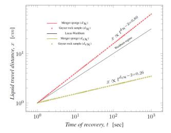
FIGURE 7. Liquid travel distance versus imbibition time in Menger sponge  $(d_{t\mathcal{H}} < d_{\mathcal{H}})$  and core samples.
