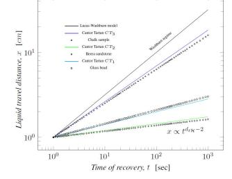
FIGURE 5. Liquid travel distance versus imbibition time in Cantor Tartan  $(d_{tH} = d_{H})$  and core samples.
