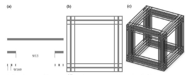
FIGURE 2. Generation process of Cantor Tartan  $CT_1$ . (a) Cantor set, i = 0, 1, 2, (b) Two-dimensional Cantor Tartan, i = 2. (c) Three dimensional Cantor tartan  $(CT_1)$ , i = 2.
