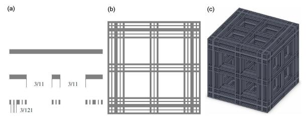
FIGURE 3. Generation process of Cantor Tartan  $CT_2$ . (a) Cantor set, i = 0, 1, 2, (b) Two-dimensional Cantor Tartan i = 2, (c) Three dimensional Cantor tartan  $\mathcal{CT}_2$ , i = 2.
