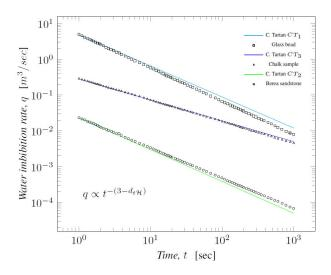
FIGURE 6. Comparison of theoretical water imbibition rate and experimental test in Cantor Tartan and core samples, respectively, where  $d_{t\mathcal{H}} = d_{\mathcal{H}}$ .
