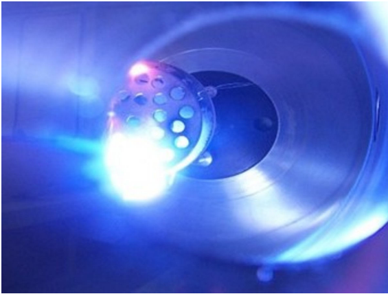
FIGURE 2. Experimental result of the spherical plasma flux from a cathodic arc discharge. The experiment was performed using a titanium cathode with combination of Argon and Nitrogen gases, and using a current of 60 A, voltage of 270 V, and a pressure of 1.7 mbar.
