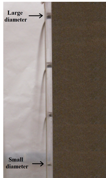
FIGURE 2. Picture of a brimful bin with beach sand in contact with a sidewall. It is observed that there are four open staggered drills on an acrylic-made (transparent) thick sidewall. The larger lateral hole allows the granular flow meanwhile for the smallest of them there is no flow, due to the condition \alpha \leq \theta_r has been reached.
