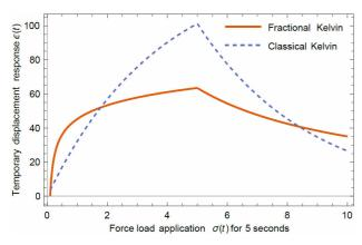
FIGURE 4. Displacement response for the Kelvin model. Fractional and integer.
