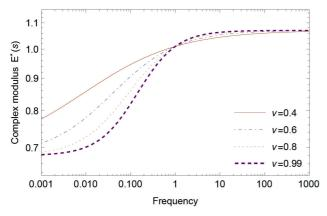
FIGURE 8. Complex modulus, observe that for values nearest to integer order one, the graphic present the traditional form.
