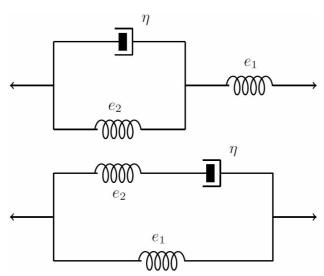
FIGURE 1. Kelvin model (KM) on top, Standard lineal solid model other known as Zener model (ZM).
