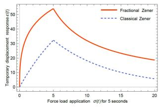
FIGURE 3. Displacement response for the Zener model (fractional and integer order), for arbitrary constant values and fractional order  $\nu = 0.4$ . The election of this value will be justify latter.
