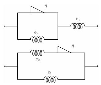
FIGURE 2. Fractional Kelvin model (FKM) on top and at the bottom Zener fractional model (FZM), can be observe that the basic idea consist in to replace the dash pot for a new element know as spring-pot.
