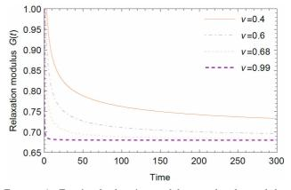
FIGURE 6. Fractional relaxation modulus, can be observed that for a near integer order,  $\nu = 0.99$  the relaxation function have an exponential behavior.
