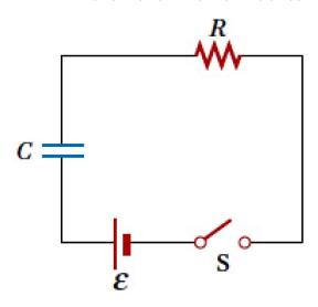
FIGURE 1. Charging a capacitor in RC circuit.
