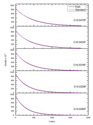
FIGURE 5. During discharging a capacitor, the changing of voltage of capacitor in the course of time for  $R=10~\rm k\Omega$  and different capacitors which are  $C=0.047~\rm F,$   $C=0.0423~\rm F,$   $C=0.0376~\rm F,$   $C=0.0329~\rm and$   $C=0.0282~\rm F.$
