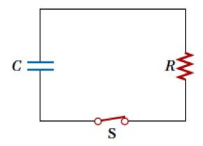
FIGURE 2. Discharging a capacitor in RC circuit.
