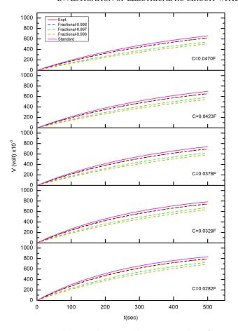
FIGURE 3. During charging a capacitor, the changing of voltage of capacitor in the course of time for  $\varepsilon=1$  V,  $R=10~\mathrm{k}\Omega$  and different capacitors which are  $C=0.047~\mathrm{F},\,C=0.0423~\mathrm{F},\,C=0.0376~\mathrm{F},\,C=0.0329$  and  $C=0.0282~\mathrm{F}$ . (The error bars have been shown with yellow).
