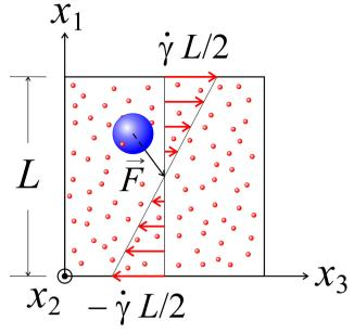
FIGURE 1.(Color online) Schematic illustration of the simulated system. The BP is represented by a big blue sphere, while solvent particles are represented by small red spheres. The application of LEBC, as it is described in the text, establishes the planar Couette flow represented by the red arrows. The harmonic force on the BP,  $\vec{F}$ , is directed towards the center of the simulation box.
