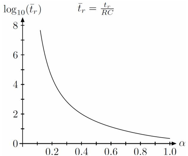
FIGURE 5. Plot of the rise time versus fractional order derivative, in the graph  $\alpha = \gamma$ .
