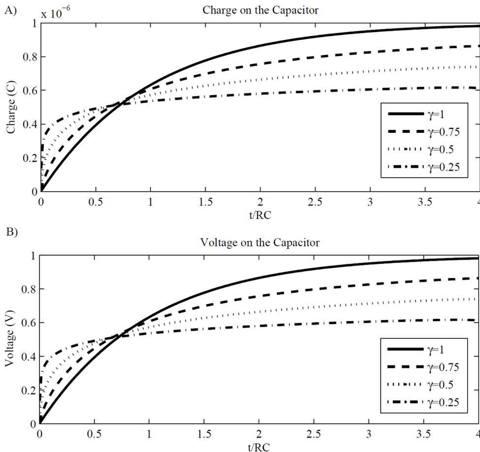
FIGURE 2. Charge on the capacitor, in Figure A), exponents:  $\gamma = 0.25, \gamma = 0.5, \gamma = 0.75$  and  $\gamma = 1$ , in Figure B), voltage on the capacitor, exponents:  $\gamma = 0.25, \gamma = 0.5, \gamma = 0.75$  and  $\gamma = 1$ .
