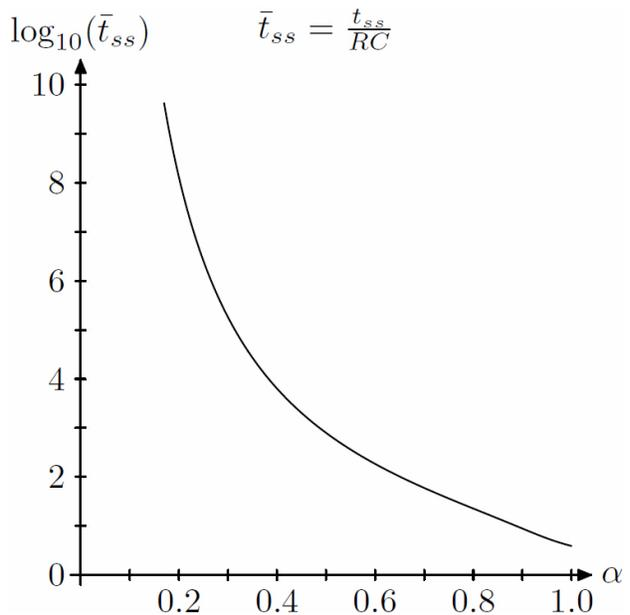
FIGURE 6. Plot of the settling time versus fractional order derivative, in the graph  $\alpha = \gamma$ .
