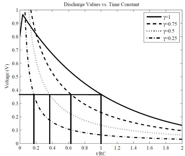
FIGURE 3. Discharge values of voltage in the  $RC$  circuit, exponent  $\gamma = 1$ ,  $\tau = 0.368$  located in  $t = 1$  second, fractional exponents:  $\gamma = 0.75$ ,  $\tau = 0.368$  located in  $t = 0.628$  seconds,  $\gamma = 0.5$ ,  $\tau = 0.368$  located in  $t = 0.369$  seconds and  $\gamma = 0.25$ ,  $\tau = 0.368$  located in  $t = 0.177$  seconds.
