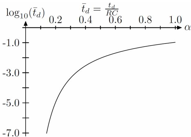
FIGURE 4. Plot of the delay time versus fractional order derivative, in the graph  $\alpha = \gamma$ .
