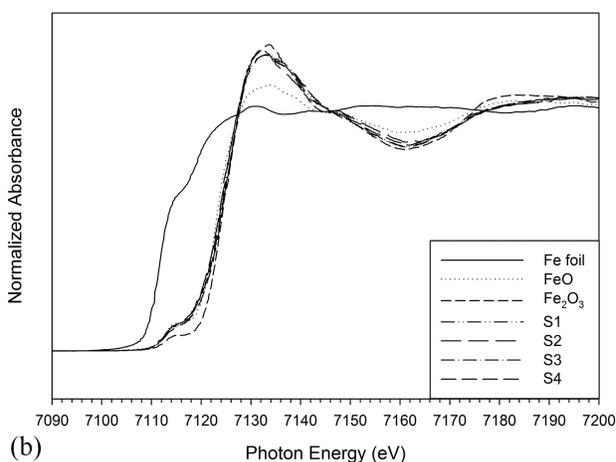
FIGURE 2. XANES spectra of as-synthesized nanoparticles (samples S1-S4); (a) Pt  $M_5$ -edge and (b) Fe K-edge.
