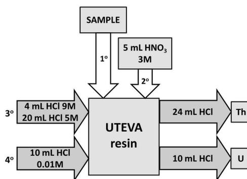
FIGURE 3. Chromatographic separation technique using UTEVA resin.
