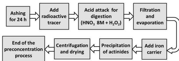
FIGURE 1. General procedure for sample digestion.
