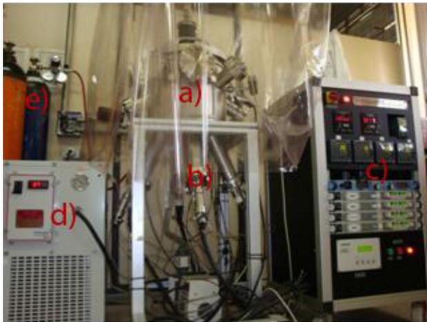
FIGURE 1. PVD deposition system: a) Deposition chamber, b) Knudsen-type effusion cells, c) General control panel, d) chiller system and e) High purity N<sub>2</sub> for venting the chamber.
