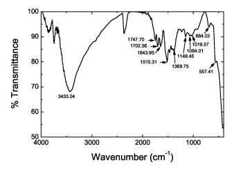
FIGURE 5. FT IR spectrum of  $\gamma$ -Fe<sub>2</sub>O<sub>3</sub>/ZnO composite particles.
