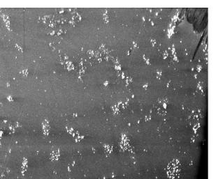
FIGURE 1. Scanning electron microscopy image of the seed magnetic  $\gamma$ -Fe<sub>2</sub>O<sub>3</sub> particles.
