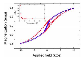
FIGURE 8. Magnetization as a function of applied magnetic field of a sample of  $\gamma$ -Fe<sub>2</sub>O<sub>3</sub>/ZnO composite, the curves were measured at 2 K (circles) and 12 K (squares). Note that the curve measured at 12 K does not show hysteresis. The inset shows the coercive field as a function of temperature.
