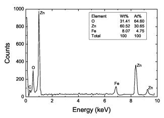
FIGURE 3. Composition and EDX of the  $\gamma$ -Fe<sub>2</sub>O<sub>3</sub>/ZnO composite.
