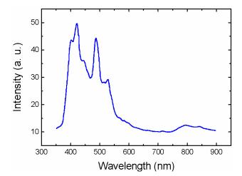
FIGURE 6. Spectrum of photoluminescence of  $\gamma$ -Fe<sub>2</sub>O<sub>3</sub>/ZnO composite particles under 358 nm excitation.
