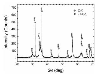
FIGURE 4. XRD pattern of  $\gamma$ -Fe<sub>2</sub>O<sub>3</sub>/ZnO composite particles. The diffraction peaks of ZnO are indicated by diamonds and the diffractions peaks of  $\gamma$ -Fe<sub>2</sub>O<sub>3</sub> are indicated by dots.
