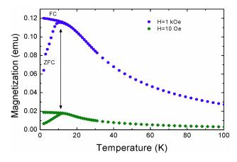
FIGURE 7. Magnetization as a function of temperature of the  $\gamma$ -Fe<sub>2</sub>O<sub>3</sub>/ZnO composite. Measurements correspond to the same sample under magnetic field of 10 Oe and 1 kOe, in the ZFC and FC mode. The arrows indicate the maximum in the ZFC curve that occurs at T=12 K.
