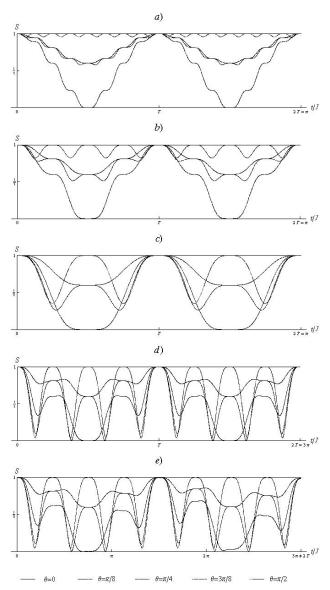
FIGURE 3. Entanglement evolution for different values of  $\theta$  and  $j = J/R \in [0, 1/2]$ . Periodic behavior is only possible for rational j: a) 1/16, b) 1/8, c) 1/4 and d) 3/8. By increasing j we increase the number of oscillations of the entropy of entanglement, while for  $\theta = \pi/4$  the maximum variation is reached in all cases. Evolution for irrational j is shown in e), with  $j = 1/\sqrt{7} \approx 3/8$ , showing a non-periodic behavior.
