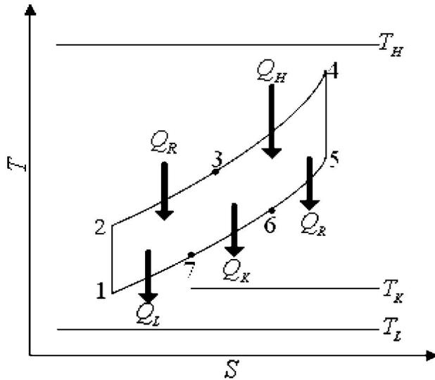
FIGURE 1. The cogeneration plant model composed of an endoreversible regenerative gas turbine closed-cycle.
