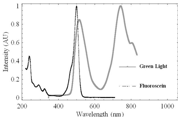
FIGURE 1. Absorption spectrum of florescein and optical spectrum of the light source used for this bonding agent.
