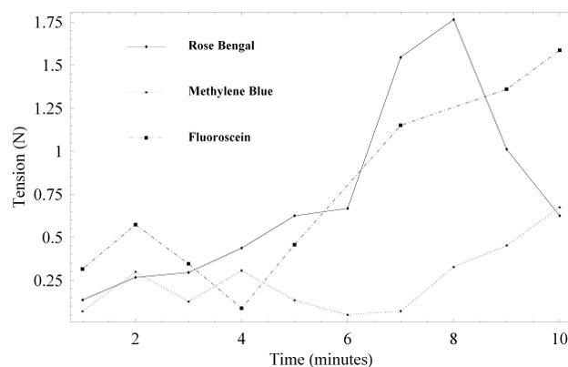
FIGURE 4. Maximum tension strength as a function of irradiation time.
