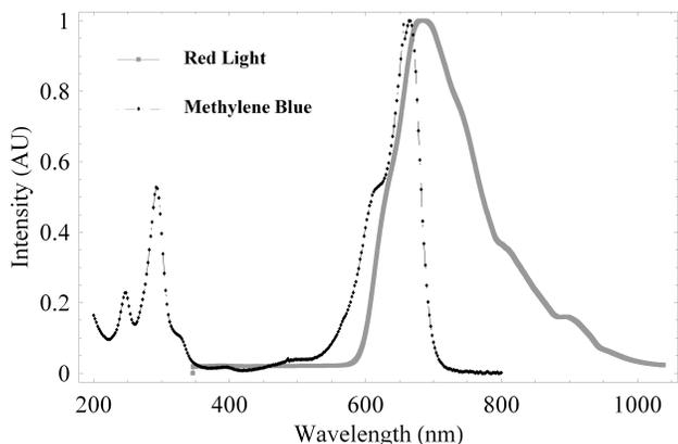
FIGURE 2. Absorption spectrum of methylene blue and optical spectrum of the light source used for this bonding agent.
