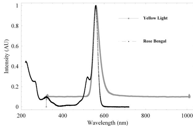
FIGURE 3. Absorption spectrum of rose bengal and optical spectrum of the light source used for this bonding agent.
