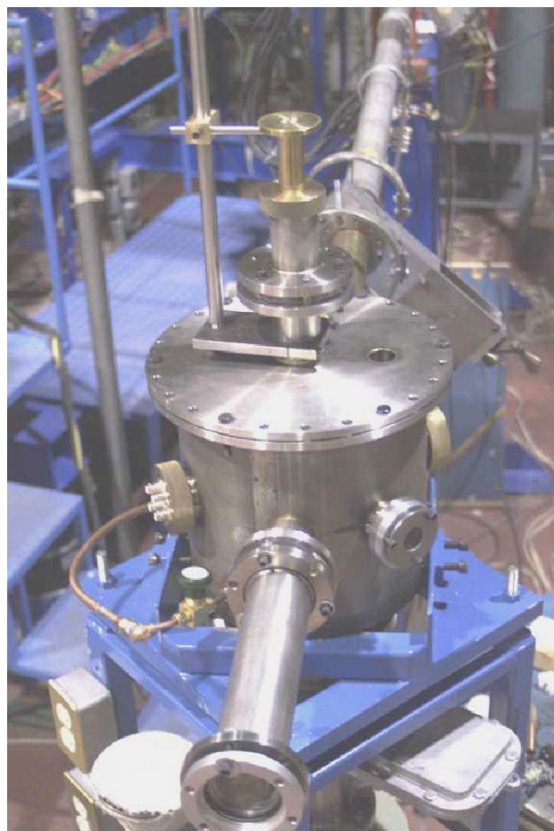
FIGURE 6. Scattering vacuum chamber used for applications of PIXE, DIXE, PIGE, RBS and NRA.
