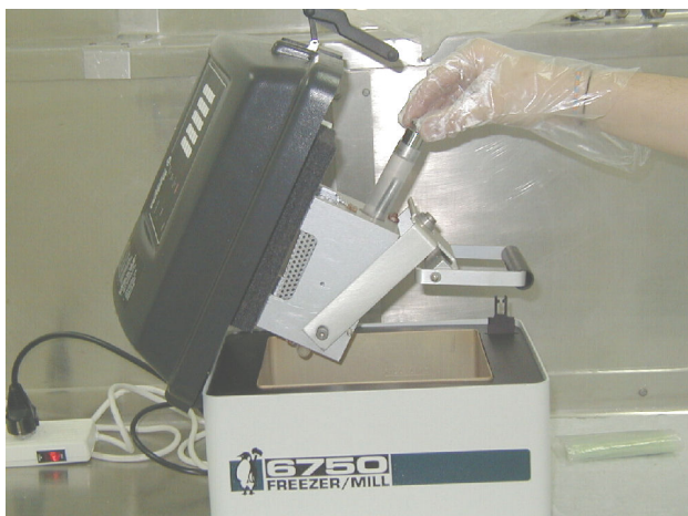
FIGURE 4. Figure shows part of sample preparation process for PIXE analysis; it is the cryogenic mill.
