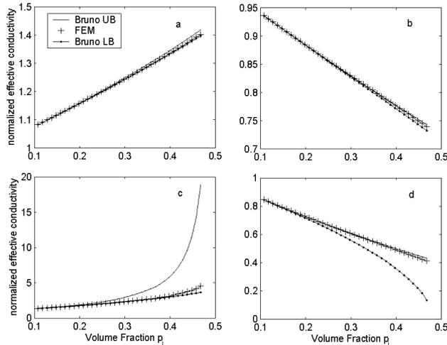
FIGURE 6. Comparison of the FEM results with Bruno's bounds for the normalized effective conductivity against inclusion volume fraction for a conducting sphere in a conducting matrix, a)  $\kappa_I/\kappa_M = 2$ , b)  $\kappa_I/\kappa_M = 0.5$ , c)  $\kappa_I/\kappa_M \rightarrow \infty$  and d)  $\kappa_I/\kappa_M = 0$ .
