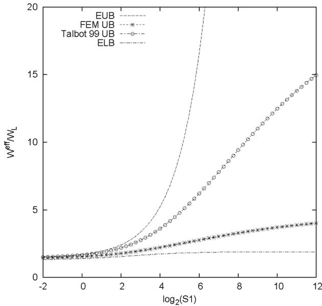
FIGURE 3. Bounds for nonlinear inclusions in a linear matrix with fixed volume fraction  $p_1 = 0.470597$ . The curves are labelled as in Fig. 1 with UB the upper bound obtained from Eq. (3).
