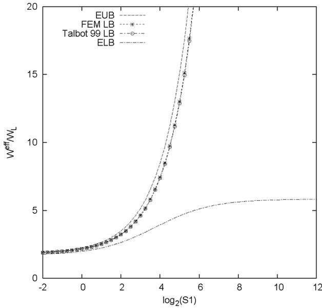
FIGURE 1. Bounds for linear inclusions in a nonlinear matrix with fixed volume fraction  $p_1 = 0.1715$ . The curves are labelled: EUB and ELB are the simple upper and lower bounds obtained in Ref. 26 by substituting constant trial fields into Eq. (1) or in its dual; Talbot 99 LB and FEM LB, are the lower bounds obtained substituting the effective property into Eq. (2) with the lower bound of Bruno and the FEM approximation, respectively.
