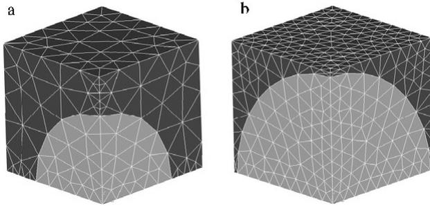
FIGURE 5. Mesh scheme for two volume fractions a)  $p_1 = 0.1715$  and b)  $p_1 = 0.470597$ .
