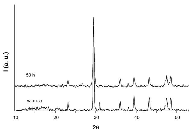
FIGURE 3. XRD patterns of limestone C1 without milling and after 50 h of mechanical treatment.
