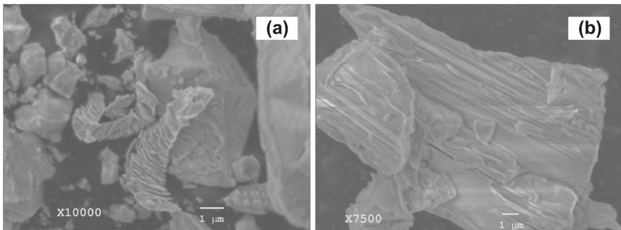
FIGURE 6. SEM micrographs of β-CaSiO<sub>4</sub> prepared by the solid state reaction of mechanically activated powders of CaCO<sub>3</sub> + SiO<sub>2</sub>. T<sub>max</sub> = 1450°C.
