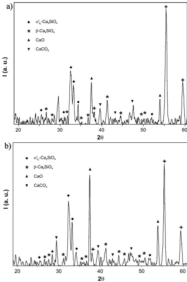
FIGURE 4. XRD pattern of the products after the solid state reaction between limestone and SiO<sub>2</sub>. T<sub>max</sub> = 1000°C. The reactants powders have been milled during 50 h, powder size (a) 105 μm, (b) 53 μm.
