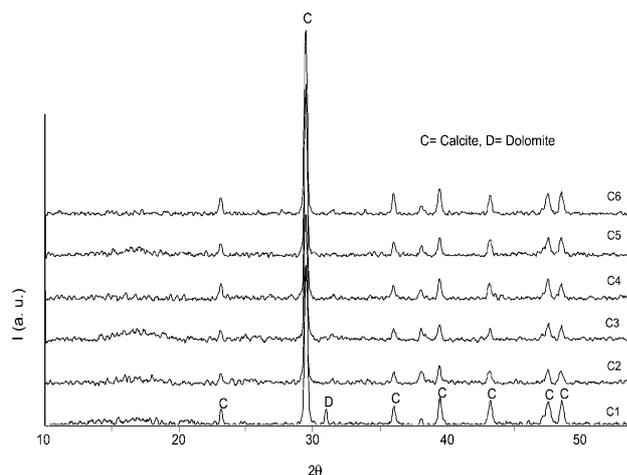
FIGURE 2. XRD patterns of several limestone after milling.
