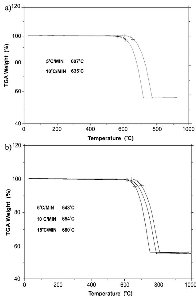
FIGURE 1. TGA curves of thermal decomposition of  $\text{CaCO}_3$  at heating rates of  $15^\circ\text{C}/\text{min}$  and  $5^\circ\text{C}/\text{min}$  in air. (a) limestone and (b) reactive grade.
