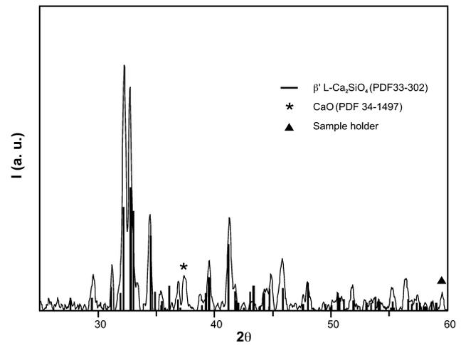
FIGURE 5. XRD pattern of the products of solid state reaction CaCO<sub>3</sub> + SiO<sub>2</sub>. T<sub>max</sub> = 1450°C, compared with PDF 33-302.
