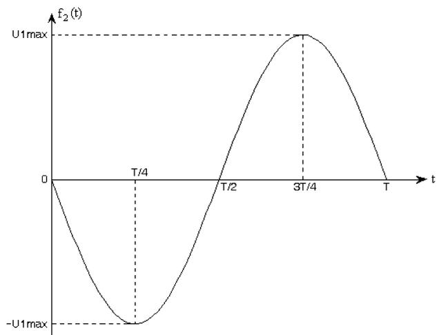
FIGURE 3. The sine voltage generated by generator  $G_2$ .
