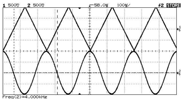
FIGURE 8. Triangular and cosine waves.
