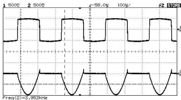
FIGURE 9. Output waves for comparator and analog switch for  $U_1=0V$ .
