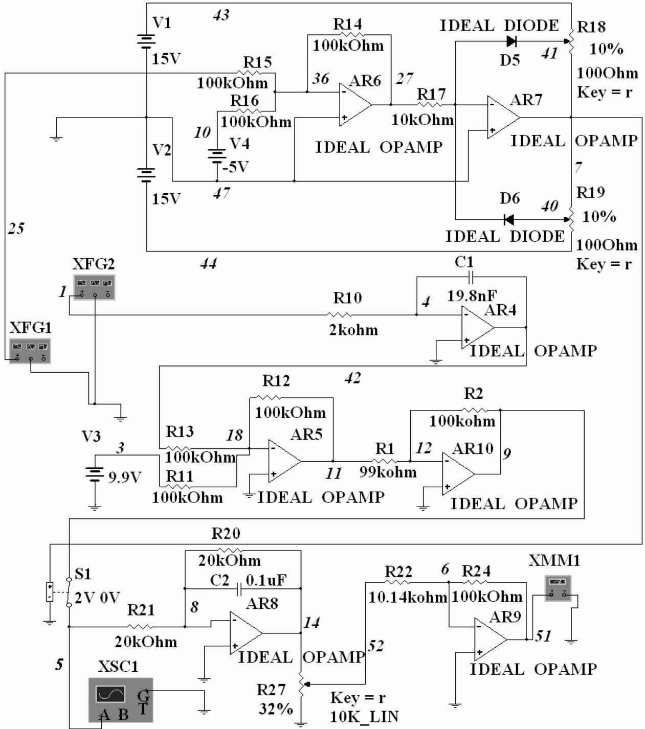
FIGURE 4. Diagram of the cosine converter.
