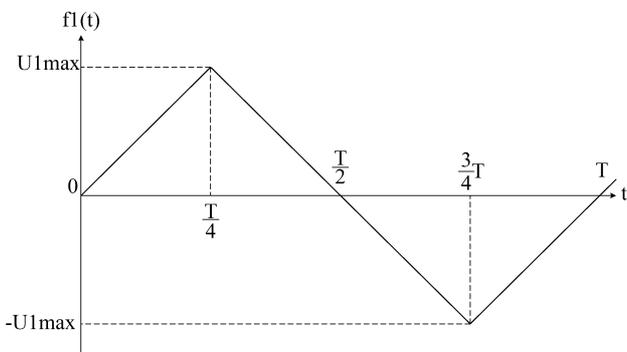
FIGURE 2. The triangular voltage generated by generator  $G_1$
