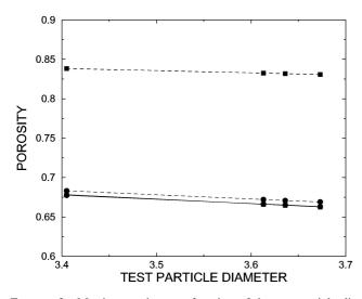
FIGURE 3. Matrix porosity as a function of the test particle diameter ( $\sigma_t$  in Å) at  $T^* = 1.5$  (solid lines) and  $T^* = 0.8$  (dashed lines) prepared with (circle) and without (square) a template. The symbols at  $T^* = 1.5$  overlap. The lines are just given as a guide.
