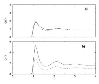
FIGURE 2. g(r) for the matrix at a)  $T^* = 1.5$  and b)  $T^* = 0.8$ . Solid lines are for matrices without a template and dashed lines for matrices with one.
