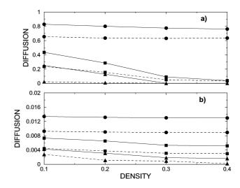
FIGURE 4. Diffusion coefficient of Ar (circle), Kr (square) and CO<sub>2</sub> (triangle) at a fluid temperature of a)  $T^* = 1.5$  and b)  $T^* = 0.8$ . The matrix was prepared without (solid line) and with (dashed line) a template at  $T^* = 0.8$ . The lines are just given as a guide.
