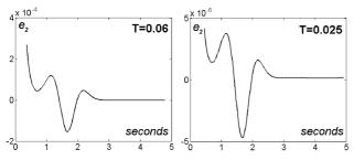
FIGURE 2. Error evolution of the second output's time derivative, for two time samplings.
