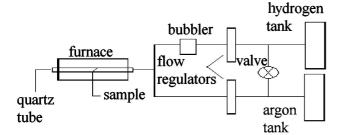
FIGURE 1. Schematic diagram of the CVD system.
