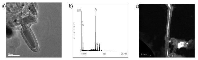
FIGURE 4. (a) Carbonaceous particle obtained with hexane at 700  $^{\circ}$ C and (b) EDS analysis showing that no oxygen is present in the core (b), the un marked peaks correspond to the copper grid of the sample holder. (c) Z-contrast image of a carbon nanotube filled with iron synthesized under the same conditions as (a).
