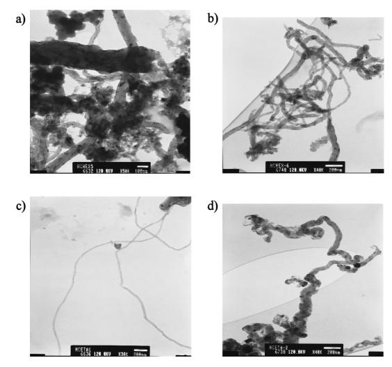
FIGURE 2. Low magnification TEM images of carbon nanotubes obtained using hexane as the carbon source at the synthesis temperature of (a)  $700^{\circ}$ C, (b)  $900^{\circ}$ C, and ethanol as the carbon source at (c)  $700^{\circ}$ C, (d)  $900^{\circ}$ C.
