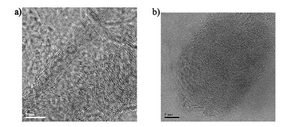
FIGURE 3. High resolution images of the multiwall carbon nanotubes obtained at  $700^{\circ}$ C, (a) from hexane and (b) from ethanol carbon sources.
