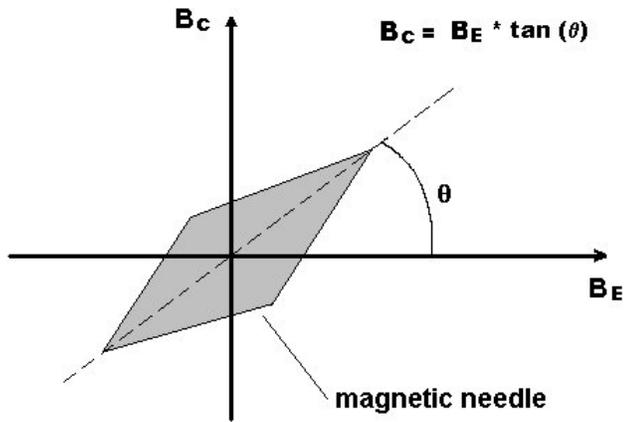
FIGURE 1. A schematic diagram of the principle of the tangent magnetometer.  $B_C$  and  $B_E$  represent the magnetic fields of both the coil and the earth. By measuring the angle of the magnetic needle it is possible to determine  $B_E$ .
