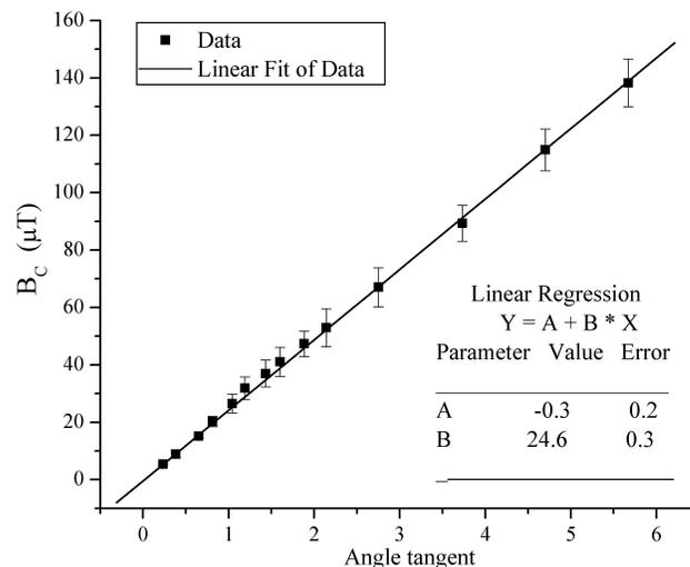
FIGURE 7. Results of the three experiments together. The uncertainties take into account the systematic errors in the experiment. The value obtained for the local earth  $B_z$  field,  $24.6 \pm 0.3 \mu\text{T}$ , agrees very well with the expected value.
