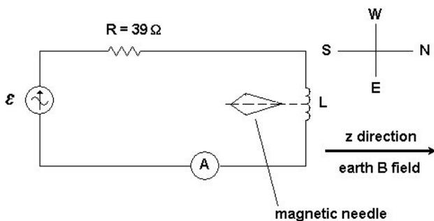
FIGURE 2. RL circuit layout employed in the experiment. The magnetic needle is oriented with its axis perpendicular to the axis of the coil, in the direction south-north of the earth magnetic field. A dc variable power source supplies a voltage from 0.1 – 3.0 V. An amperimeter in series register the current through the circuit.
