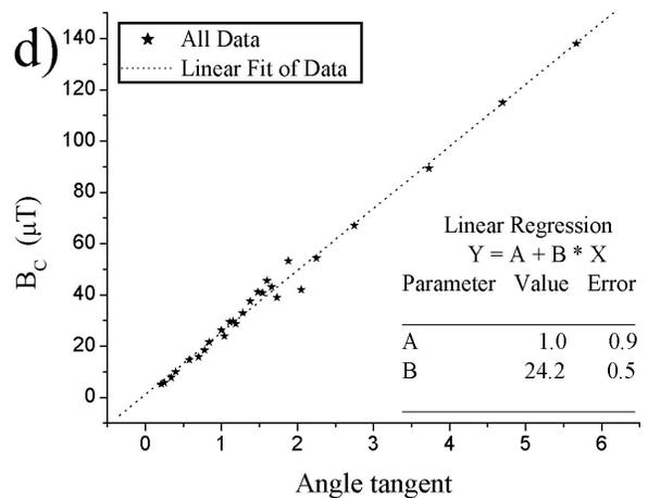
FIGURE 5. Results of (a) the first, (b) the second and (c) the third experiment, respectively. The slopes of the linear fits give the values of the local earth  $B_z$  field. (d) All of the data together.
