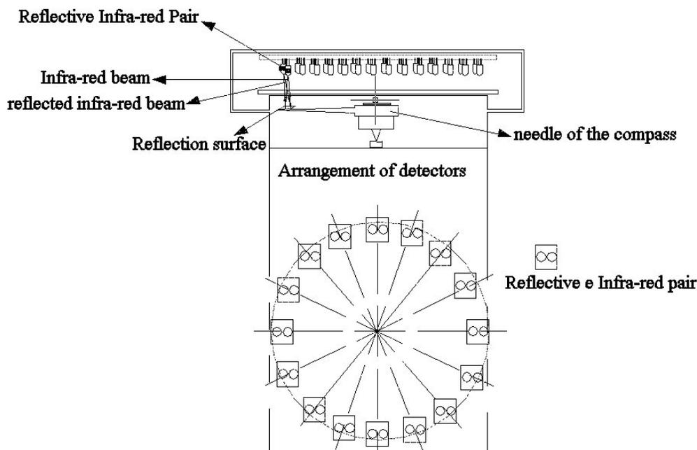
FIGURE 6. A system composed of a set of photodiodes in a circular arrangement, proposed as an alternative to measure the deflection angle on the needle of the compass. Depending on the photodiode activated the position of the needle is indicated.
