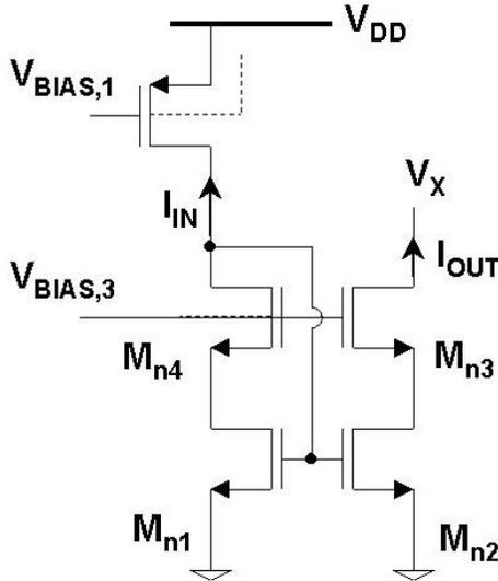
FIGURE 1 The advantage of using a cascode current mirror allows the designer to develop complex systems just cascading basic cells. It is easy to demonstrate that the impedance ratio, defined as  $Z_{in}/Z_{out}$ , is lower than 0.01% that is a recommended value for analogue signal processing.
