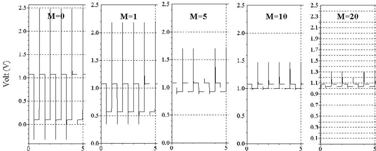
FIGURE 3 Tspice simulation result in which a NMOS capacitor has been designed with an area  $M$  times greater than  $M_{n1}$  area. The voltage variation  $\delta_{feedthrough}$  was really decreased as area increases in value. The analysis was done using a sampling frequency of 1 MHz.
