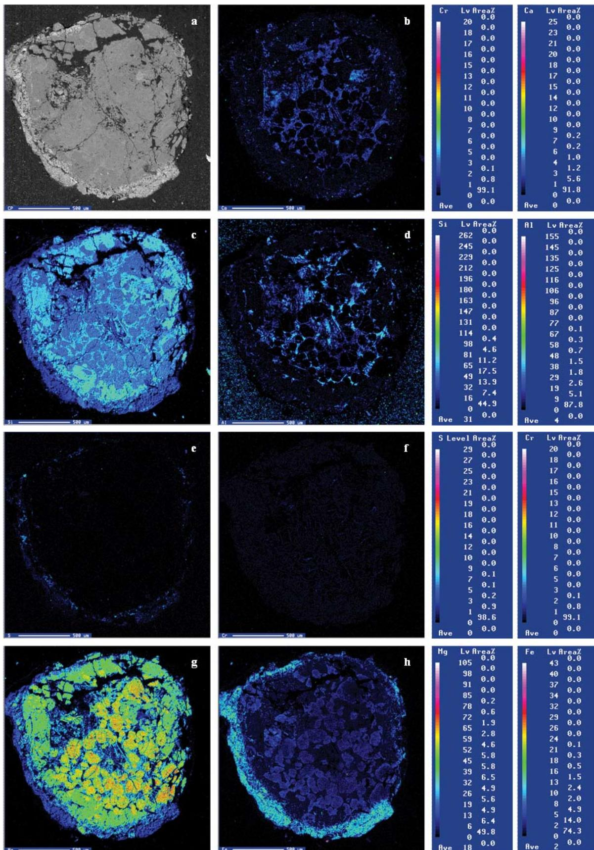
Figure 7. a: Scanning electron microscope images for chondrule M27 with scan elemental data for b: Ca, c: Si, d: Al, f: Cr, g: Mg, and h: Fe.
