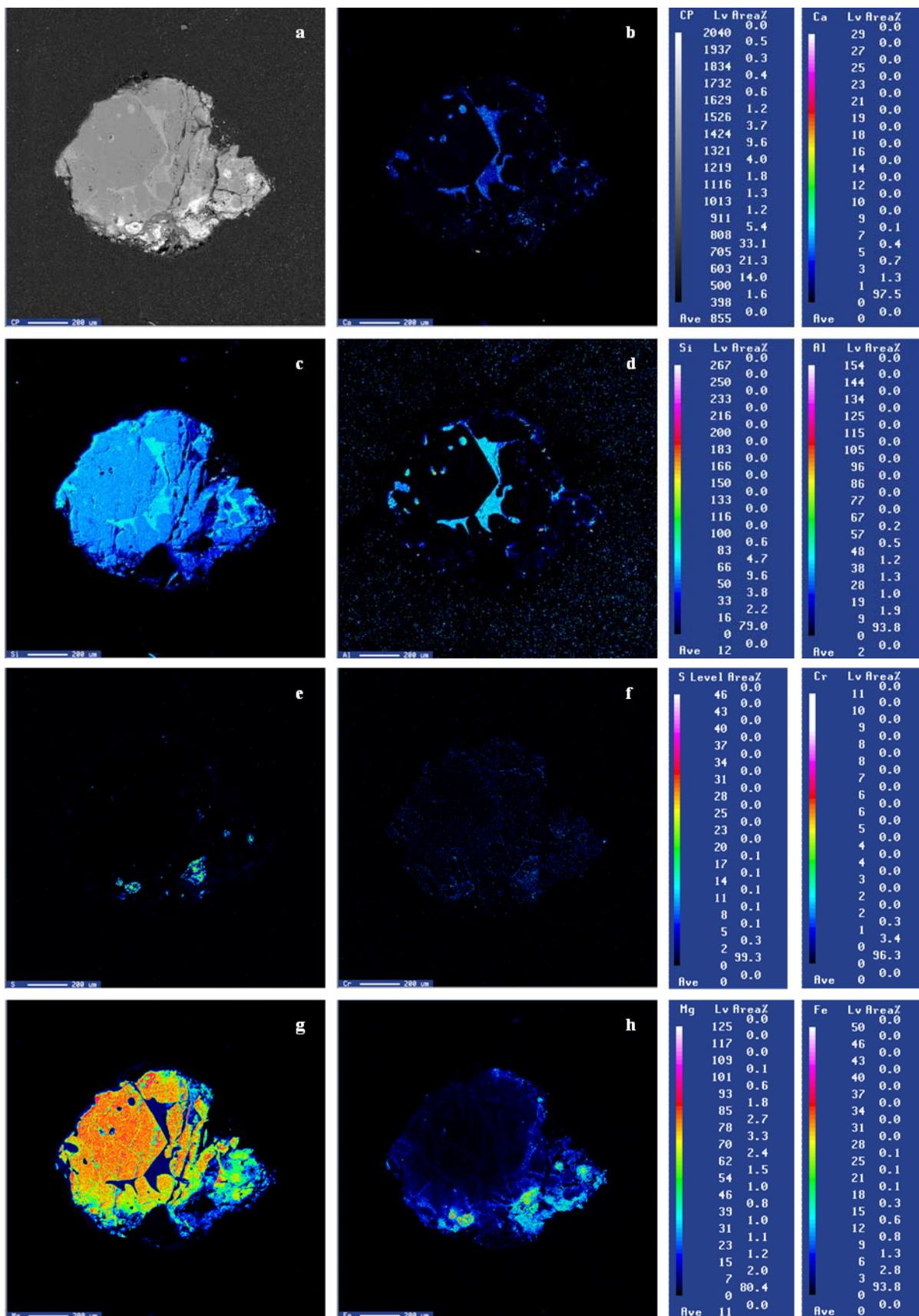
Figure 9. a: Scanning electron microscope images for chondrule M23 with scan elemental data for b: Ca, c: Si, d: Al, f: Cr, g: Mg, and h: Fe.
