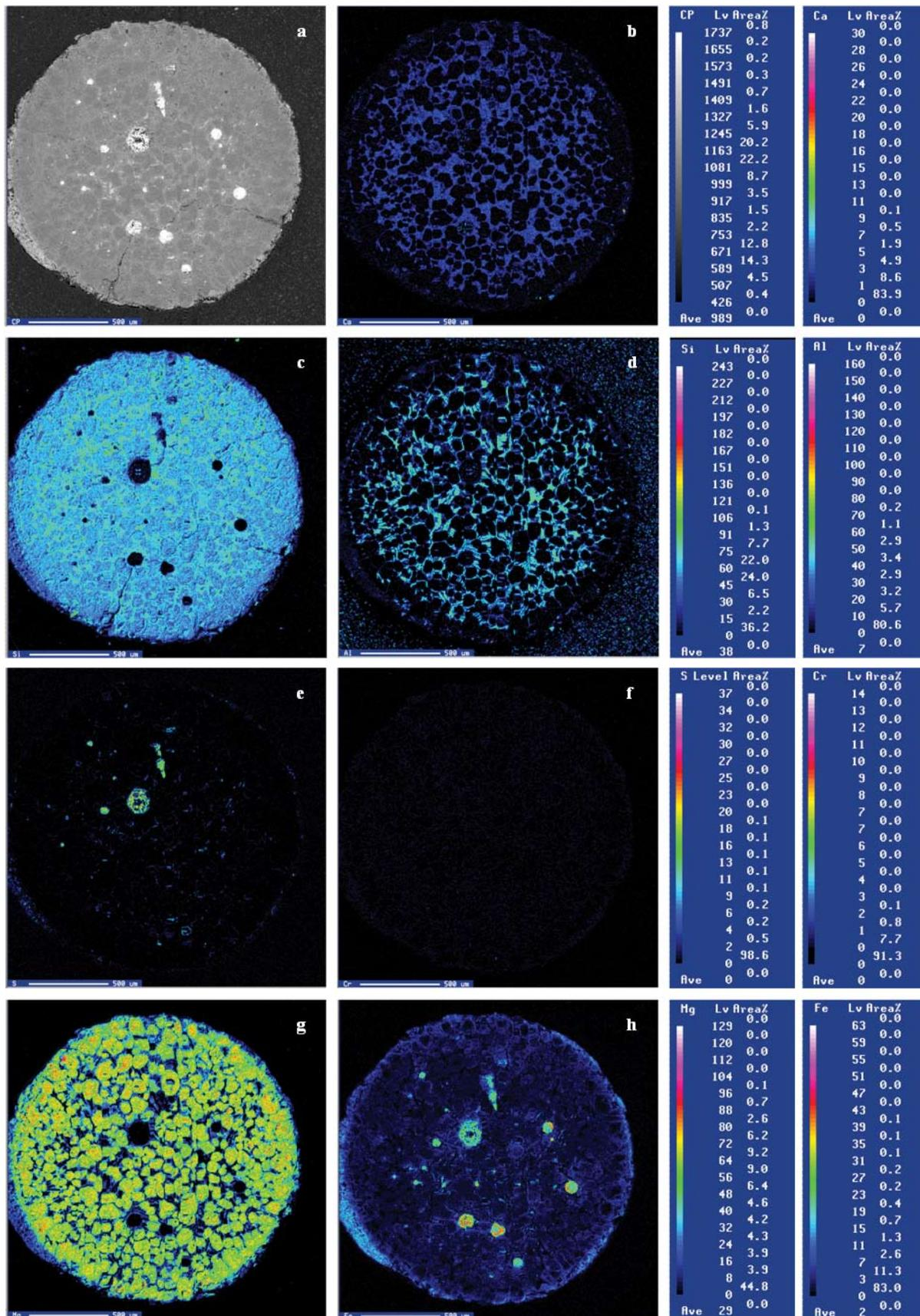
Figure 5. a: Scanning electron microscope images for chondrule M53 with scan elemental data for b: Si, c: Ca, d: Al, e: S, f: Mg, g: Cr, and h: Fe.
