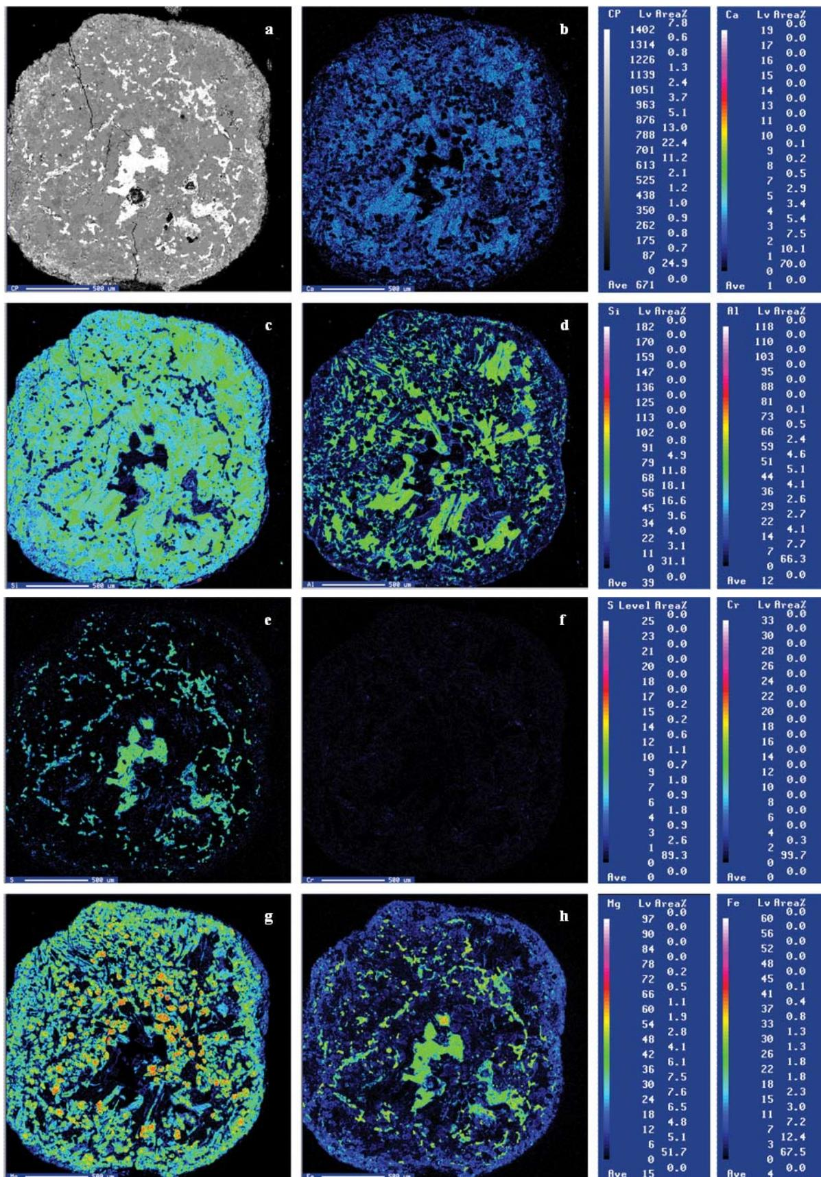
Figure 6. a: Scanning electron microscope images for chondrule M55 with scan elemental data for b: Ca, c: Si, d: Al, f: Cr, g: Mg, and h: Fe.
