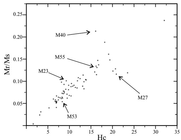
Figure 2. Plot of the magnetization ratio ( $M_r/M_s$ ) as a function of coercivity ( $H_c$ ) for individual chondrules from Allende. Note the linear trend for  $H_c$  less than 17 mT with  $M_r/M_s$  up to 0.17. Chondrules analyzed for internal microstructure are marked, covering the range of coercivity and magnetization characteristics.
