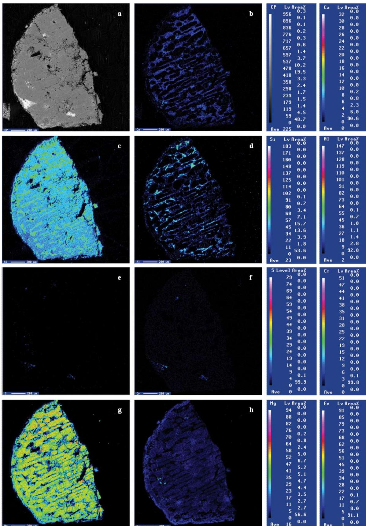
Figure 8. a: Scanning electron microscope images for chondrule M40 with scan elemental data for b: Ca, c: Si, d: Al, f: Cr, g: Mg, and h: Fe.
