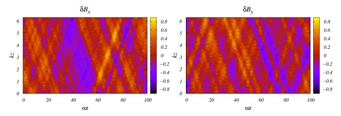
Fig. 3. Intensity plot of a particular turbulent magnetic field realization of plane waves traveling in the Z-direction at different times. The X-component is shown in the left figure while the Y-component in the right one. The total field variance here is  $\langle \delta B^2 \rangle = 1$  and  $\gamma = 2$ . Units are arbitrary. The color figure can be viewed online.
