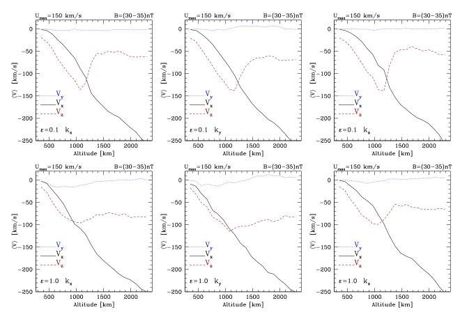
Fig. 9. As in Figure 7 but with a stronger  $B_{\min} = 30$  nT and lower  $U_{\max} = 150$  km s<sup>-1</sup> in order to favor an increase in the curvature of the O<sup>+</sup> pickup ions and its  $V_x$  component. Note that the general behavior of the profiles does not correspond to the ASPERA-3 measurements.
