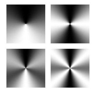
Fig. 8. Density plot of  $P_l(\cos \gamma)$ , where  $\gamma$  is the angle measured from the upper vertical direction towards both left and right. Top left: l = 1; top right: l = 2; bottom left: l = 3; bottom right: l = 4. Darker zones correspond to higher values; brighter zones to lower values.
