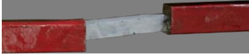
Figure 11. State of deformation of the device under severe inelastic demands (after the end of test 4)
