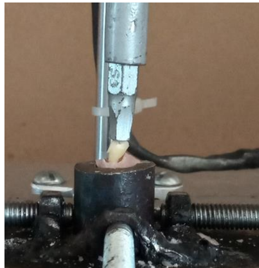
Figure 8. Push and put test performed by the prototype.
