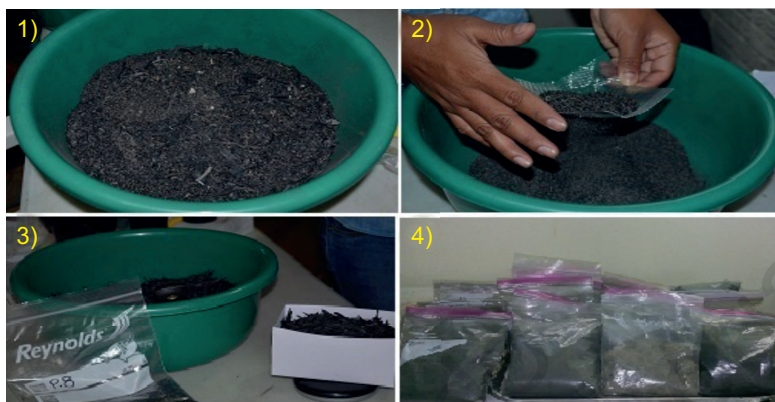
Fig. 2. Processes of: (1) collection, (2) sieving, (3) weighing, and (4) packaging of ash samples at the 51 selected sites
