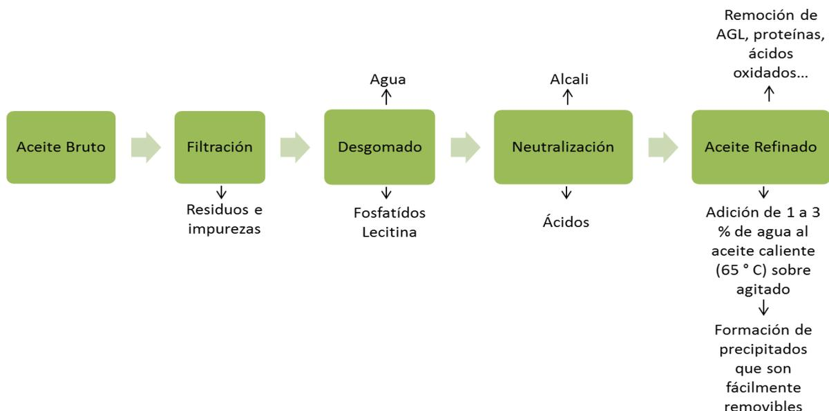
**Figure 5. Moringa oil refining process.**
