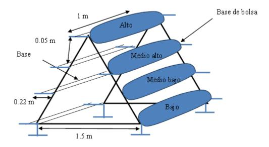
Figure 1. Diagram of the pyramidal hydroponic module, with the structure and horizontal bags located in four layers.
