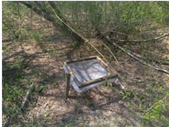
Figure 3. Mesh basket used to collect leaf litter at the TTS site (October, 2011).
