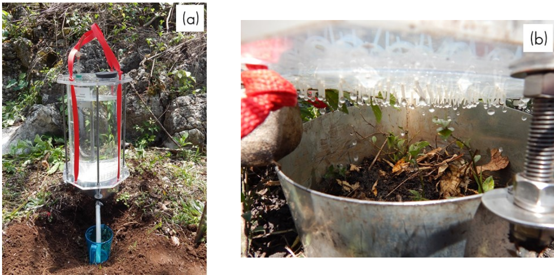
a) Infiltrrometer installed in the study site; b) Detail of the interior of a runoff measurement plot.
