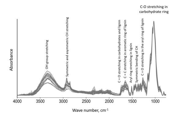
**Figure 1.** ATR-FTIR spectra of the 27 *Pinus* tablets that comprise the spectrotheque, with the assignment of the main bands.
