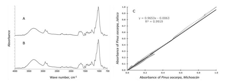
**Figure 3.** ATR-FTIR spectra of *Pinus oocarpa* Schiede woods from *Michoacán* (A) and *Jalisco* (B); C) Comparison of the absorbances between the spectra.
