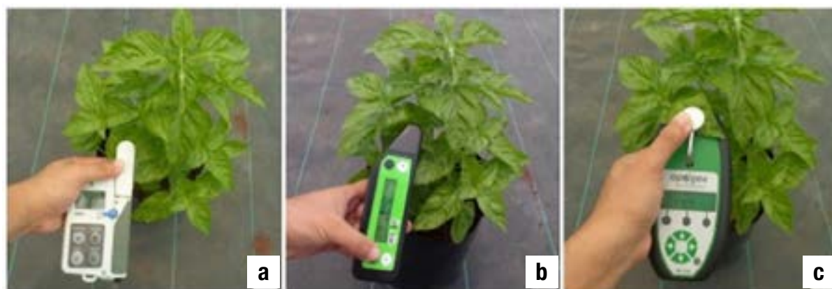
Figure 1. Use of SPAD 502 Plus (a), atLEAF (b) and MC-100 (c) to measure relative chlorophyll concentration in basil 'Nufar'.
