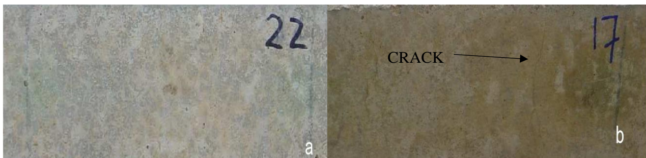
Figure 6. Beams without initial chloride contamination, rained with chlorides in the 25-cm central zone (a) non-preloaded (b) preloaded
