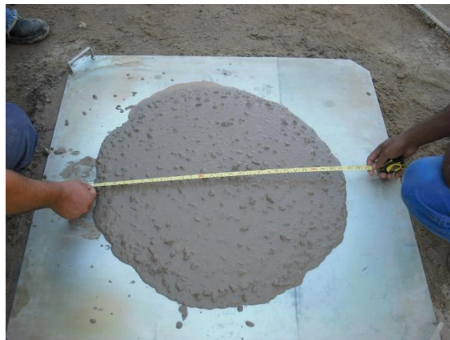
Figure 9. Measurement of concrete flow.
