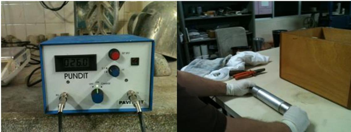
Figuras 3 – (A) e (B). Equipamento e calibração PUNDIT (Portable Ultrasonic Non-destructive Digital Indicating tester)
