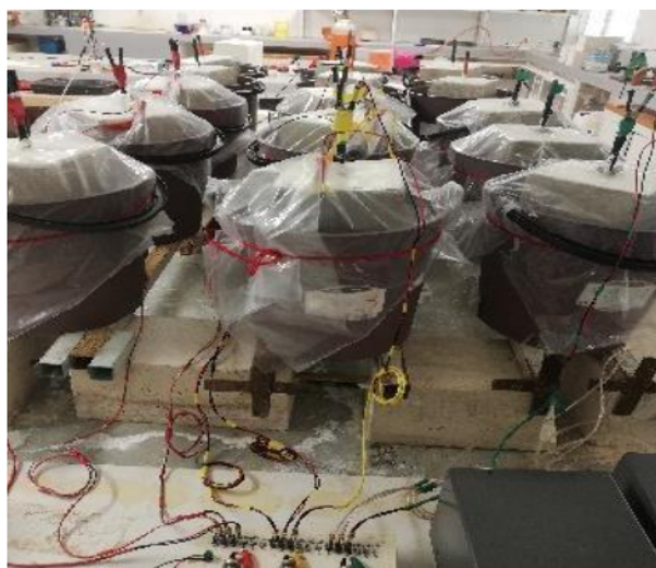
Figure 2. Experimental setup used for electrochemical re-alkalinization.
