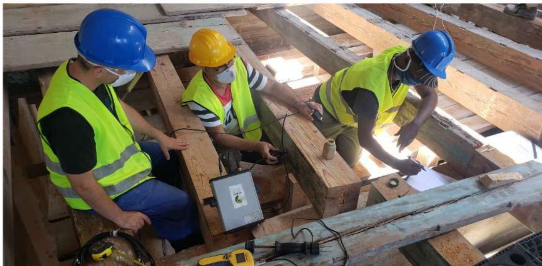
Figure 9. Application of UPV tests on wooden beams
