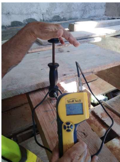
Figure 11. Surface moisture measurement with Delmhorst's TotalCheck thermo-hygrometer equipment
