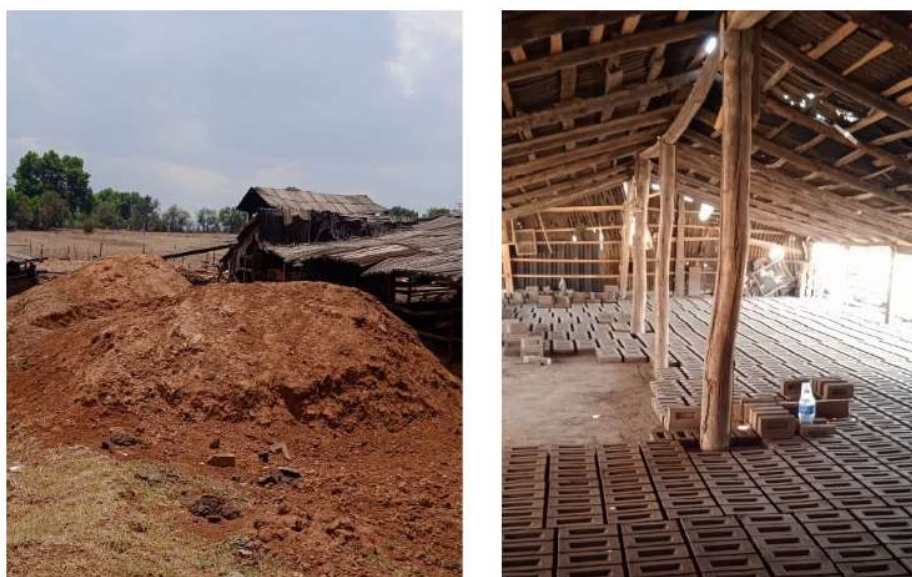
Figure 3. (a) Quarry with clayey soils in Santiago Undameo; (b) Manufacturing of ceramic and earthen construction components.
