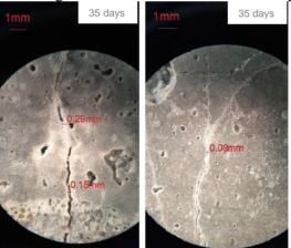
Figure 8. Self-healing in formulation SS – Samples 1 and 2.
