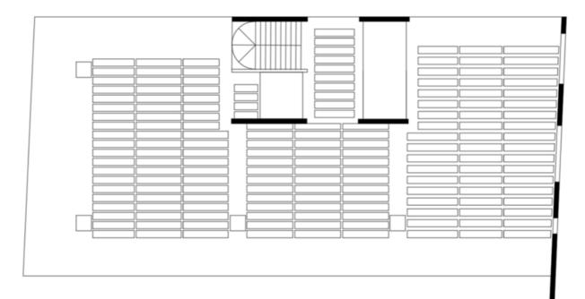
Figure 7. Grid Slab Scheme (Source: FAU-USP)
