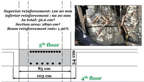
Figure 12. Configuration of the strip-beam reinforcement.
