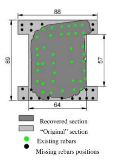
Figure 11. Reconstitution of the cross section of the recovered rubble column.
