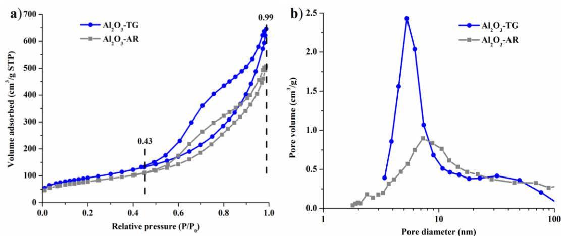
**Figure 5.** a) N<sub>2</sub> adsorption–desorption isotherm and b) pore size distribution curve of Al<sub>2</sub>O<sub>3</sub>-TG and Al<sub>2</sub>O<sub>3</sub>-AR.
