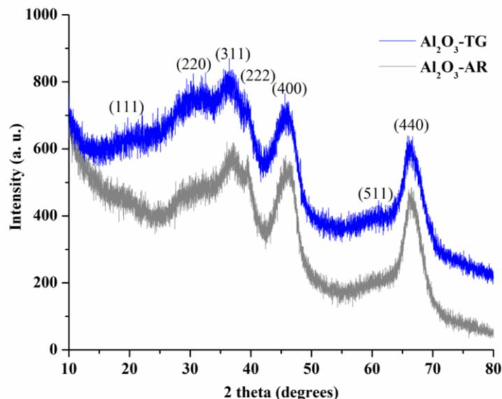
**Figure 4.** XRD patterns of a) Al<sub>2</sub>O<sub>3</sub>-TG and b) Al<sub>2</sub>O<sub>3</sub>-AR.
