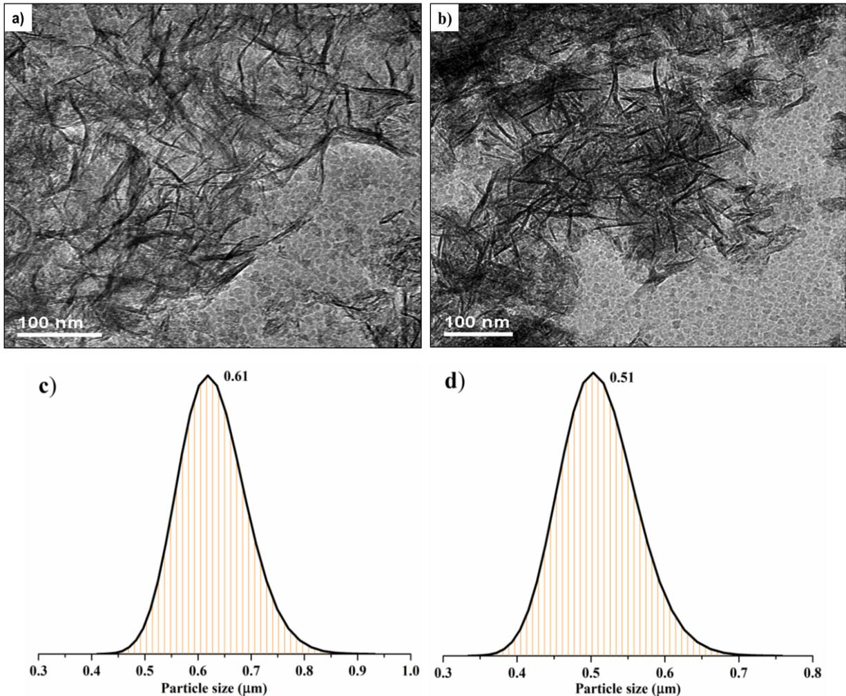
**Figure 2.** TEM images of a) Al<sub>2</sub>O<sub>3</sub>-TG, b) Al<sub>2</sub>O<sub>3</sub>-AR and particles size c) Al<sub>2</sub>O<sub>3</sub>-TG, d) Al<sub>2</sub>O<sub>3</sub>-AR
