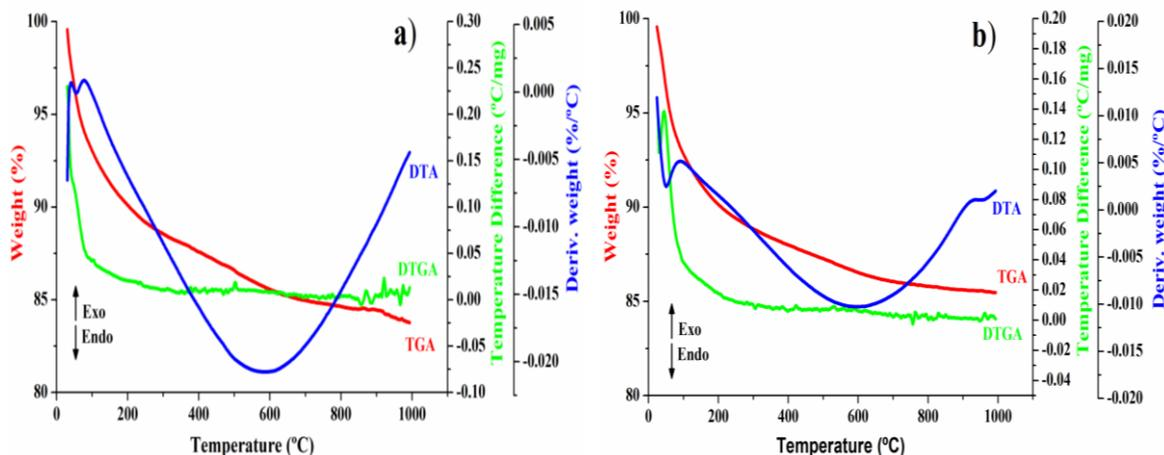
**Figure 3.** TGA/DTGA and DTA curves of a) Al<sub>2</sub>O<sub>3</sub>-TG and b) Al<sub>2</sub>O<sub>3</sub>-AR.
