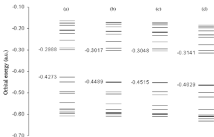
Fig. 7. Energetic behavior of highest occupied molecular orbitals and lowest unoccupied molecular orbitals for the model of two guanidinium groups, (a) without SIC correction, (b) AS-SIC including only the HOMO in the active space, (c) AS-SIC with an active space defined by the five highest occupied molecular orbitals, and (d) with an active space defined by the ten highest occupied molecular orbitals. The eigenvalues of HOMO and LUMO are reported explicitly in atomic units.
