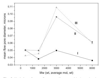
Fig. 3. Variation of mean flow pore diameter with the molecular weight of PEG in gelation bath (I. 0.5%, II. 1% and III. 2%).
