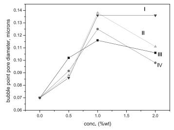
**Fig. 2.** Variation of Bubble point pore diameter with the concentration of PEG in gelation bath (I. PEG 6000, II PEG 3000, III PEG 400 and IV PEG 1500).
