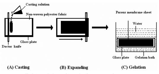
Fig. 1. Schematic diagram of preparation of porous asymmetric membrane.
