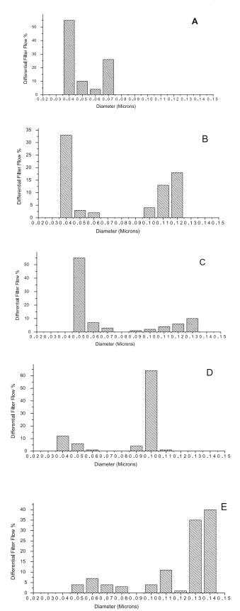
**Fig. 4.** Histogram of differential filter flow (%) with the pore diameter of the membranes (A: in water, B: in PEG 400, C: in PEG1500, D: in PEG 3000, E: in PEG 6000).
